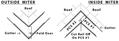
**End cap installation** To make "end-caps" or cap the ends of the gutter guard at the end of a gutter.
